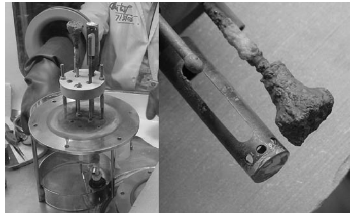
Fig. 3: Electrorefining cell and the deposit of plutonium on solid cathode
